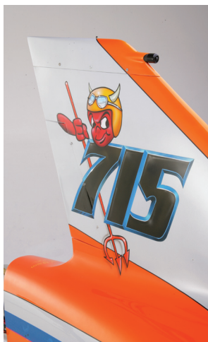
> Above: Speed Demon has a servocontrolled tail rudder that can be clocked to any degree to add stability, depending on wind conditions.
